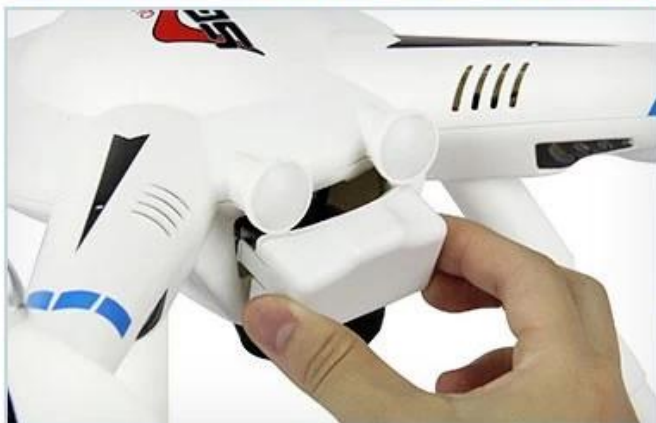
STEP 1 Hold the battery cover and pull out
