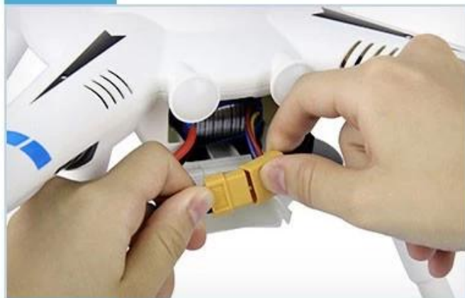
STEP 3 Connect the battery and the power wires
