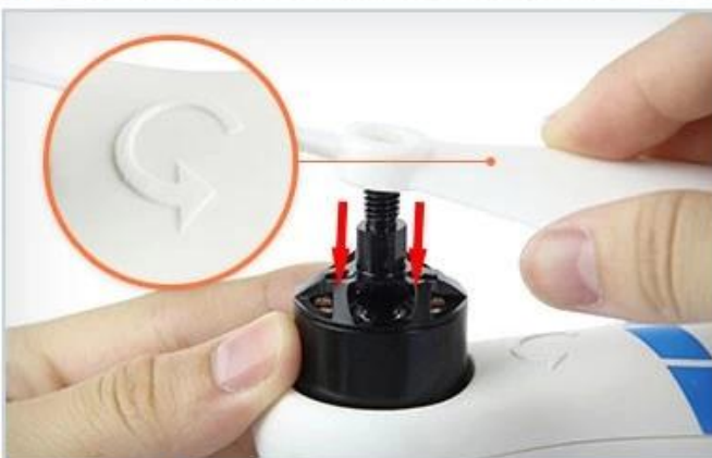
STEP 2 Make sure the rotating direction of the blades should be the same as the rotating direction of the motor
