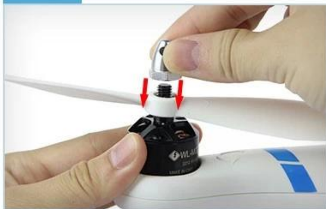
STEP 3 Put the propeller hoop on the blade
