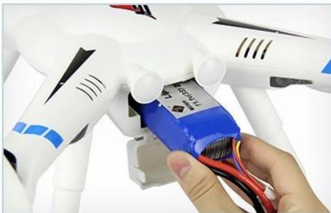
STEP 2 Put the battery into battery compartments
