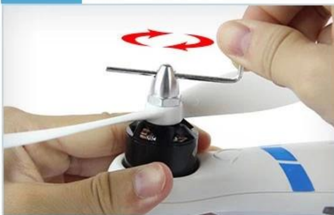
STEP 4 Insert one round stick into the hole of the propeller hoop, Reverse rotation arrow
