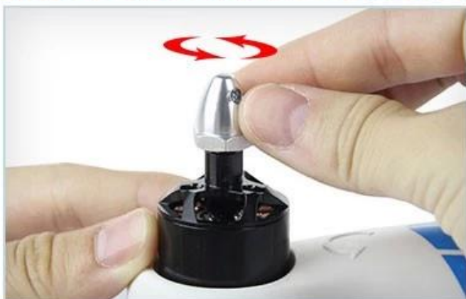
STEP 1 Take down the propeller hoop on the motor first
