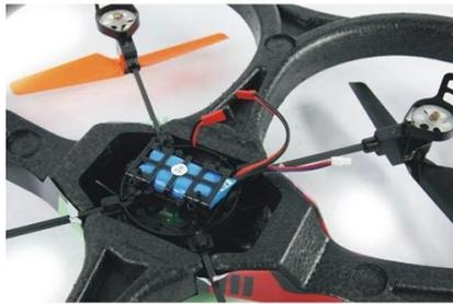
**7.4V 650MAH Li-po Battery**
