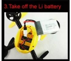
Product battery: 3.7V 300MAH Lipo battery(including) Transmitter battery: 6\*1.5V AA battery(not including)
