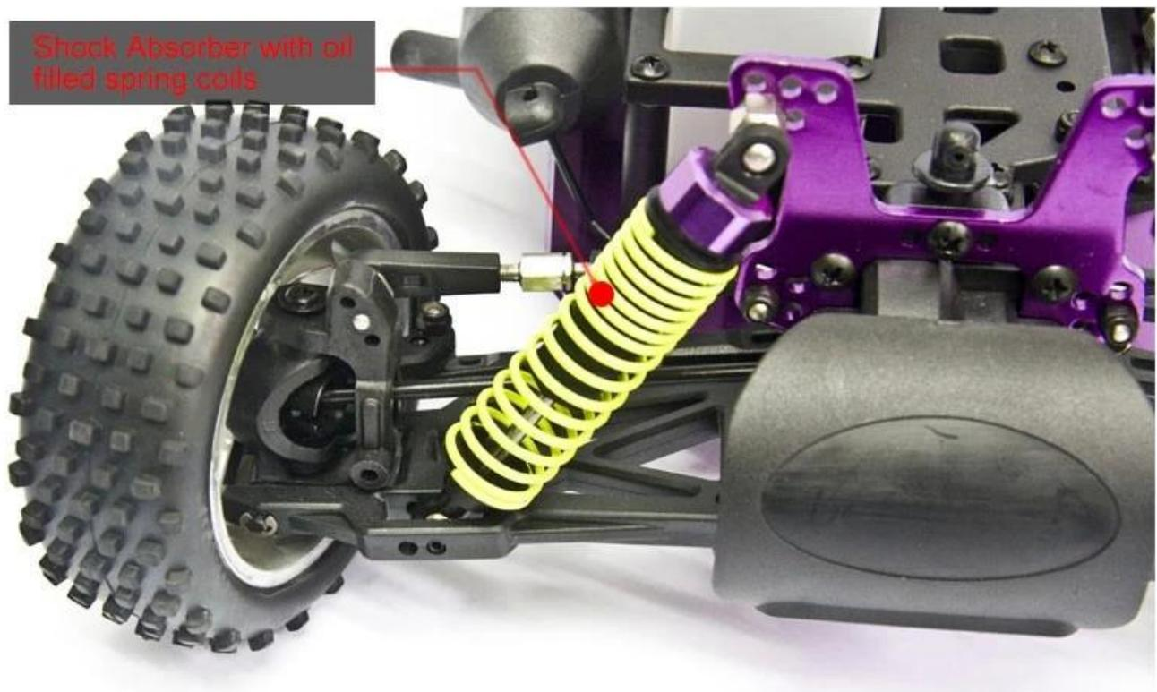
Shock Absorber with oil filled spring coils
