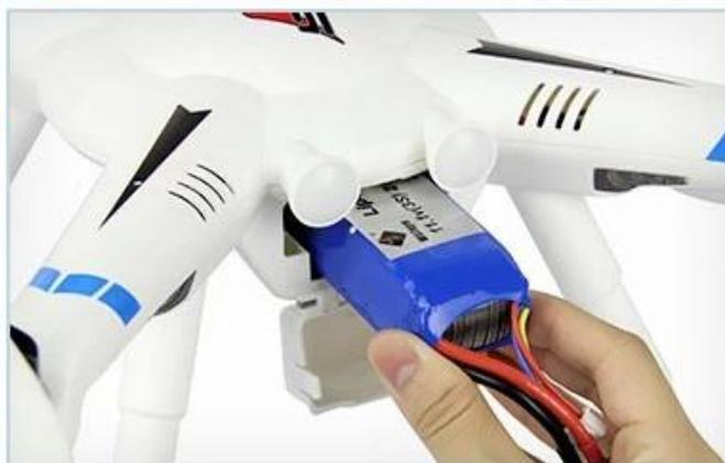
**STEP 2** Put the battery into battery compartments
