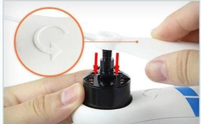
**STEP 2** Make sure the rotating direction of the blades should be the same as the rotating direction of the motor
