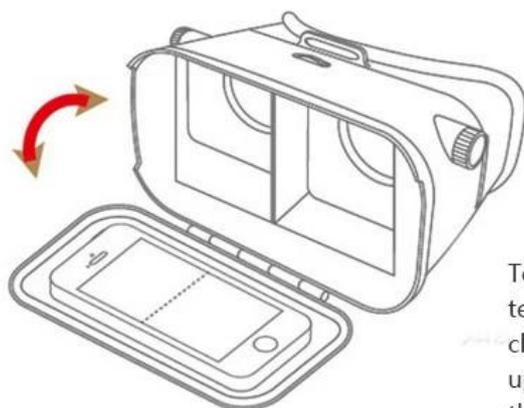
Towards the phone screen, gently struck telescopic adjustment slot, put your phone, close the cover plate (left), found the picture upside down, you can adjust the direction of the phone.
