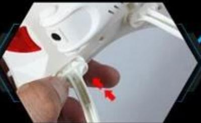
Fit the camera bottom plug socket at the bottom of the craft, and lock the camera. Then connect the cable to the camera.
