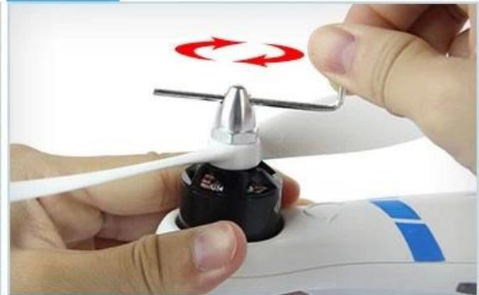
**STEP 4** Insert one round stick into the hole of the propeller hoop, Reverse rotation arrow
