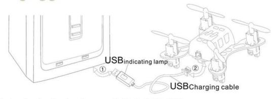
(before charging, the aircraft power switch to the "OFF" state)
